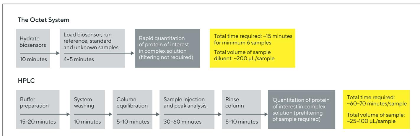
Figure 1: Illustration depicting the screening workflow in the Octet system and the HPLC system.
